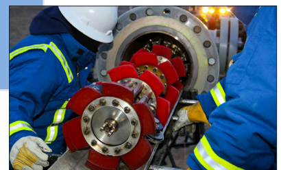
Pipelines deliver massive amounts of crude daily and ensuring safe operation is key. The EMCORE TAC-450, coupled to additional sensors, provides these inspection robots with extremely accurate angular data.
