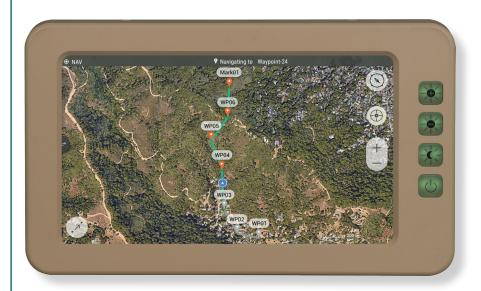
The EMCORE Moving Map Display (MMD) delivers real-time tactical moving map technology, displaying internally stored maps with a moving icon indicating vehicle location, as well as other pertinent navigation information. Users can create, store, and activate waypoints and routes from the touchscreen, which is viewable in all lighting conditions.
