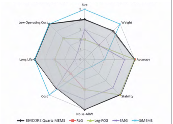
FIGURE 1: EMCORE QMEMS Inertial Sensor Technology Points of Difference for Tactical Applications
