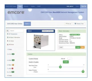
The OPV-CTLR-X-IC Controller Card can serve as an interface providing critical data to any SNMP based Management Software, such as HP Openview Source and showing the connect/disconnect for data signals, ensuring both independence and flexibility in system management. Also, by knowing the health of each remote card, the client can save trips to the install facility and manage switching to a back-up card through the software.
