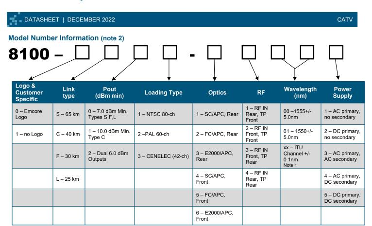
Note 1: ITU grid wavelengths can be specified from channel 18 to 62. Contact factory for availability
