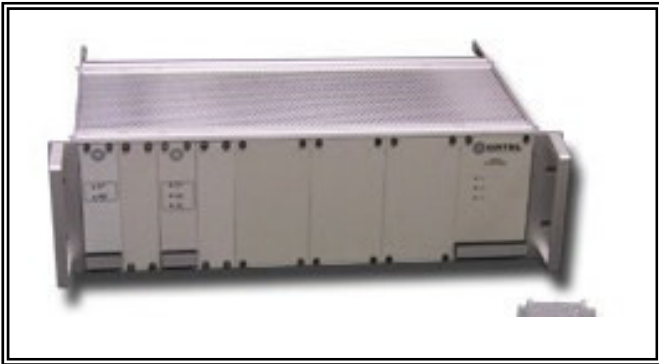
Figure 9. Rack Mountable Fiberoptic Delay Line. The unit shown here is 10 GHz, 280 microsecond delay. The RF input and output connectors are standard SMA.
