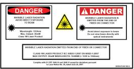
Caution: Use of controls, adjustments and procedures other than those specified herein may result in hazardous laser radiation exposure. \*IEC is a registered trademark of the International Electrotechnical Commission.
