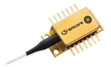
EMCORE's 1782 laser module is characterized for use as a CW optical source in CATV and DWDM networks. The 1782 is dc-coupled with a built-in TEC, thermistor, and monitor photodiode. The device is mounted in a 14-pin, OC-48 pinout compatible butterfly package with the optical isolator mounted on the TEC. The 1782 incorporates a high efficiency coupling scheme to deliver 40 mW, 50 mW, 63 mW, 80 mW and 100 mW of CW optical power.
